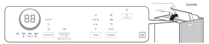
Open the louvres manually before operation. (After operation is stopped, louvres are not closed automatically because it is hand-operated)
